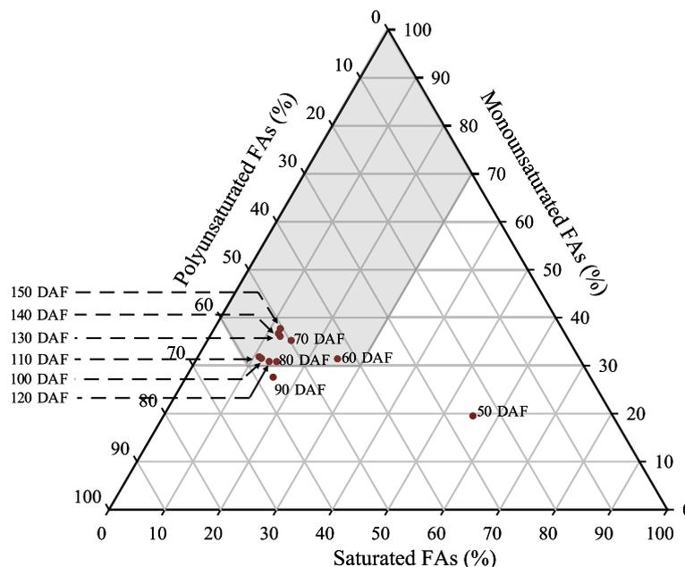
**Fig. 7** Placement of kernel oil samples on a chart predictive of biodiesel properties based on FA composition. The gray area delineates FA compositions satisfying limits for biodiesel fuel properties
