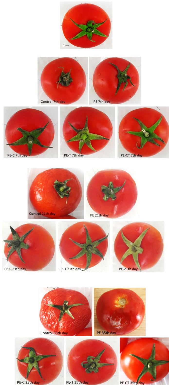
Fig. 10 The appearance of tomato fruit during 42 days storage at 4 °C. PE (neat LDPE), PE-C (nanocomposite film containing 3% clay nanoparticles), PE-T (nanocomposite film containing 3% TiO 2 nanoparticles), PE-CT (nanocomposite film containing 3% TiO 2 and 3% clay nanoparticles), control (unpacked tomato fruits)
